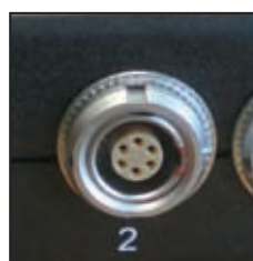
Input Connectors Highest quality latching metal 'Lemo' connectors.
